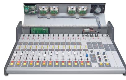
**THE MIDSIZE R-55E MAINFRAME** (shown here with optional phone, second studio and line selector modules) comes standard with twelve inputs (13 max) and four mic preamps (8 max). Note how the R-55E hinged meterbridge swings up and open for easy access to I/O connectors, logic programming dipswitches and calibration trimpots.
