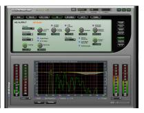
AM-10HD setup and processing adjustments are done via the Vorsis Control Software, PC software installed on your computer, either locally at the AM-10HD or remotely over WAN or the Internet.
