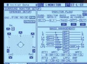
SURROUND MONITOR SETUP (THX pm3™ MONITOR FLOW)
