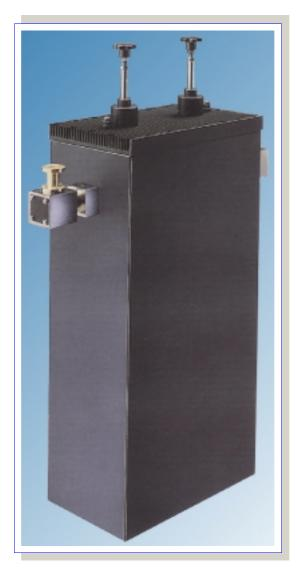
THE DCF ARE ONE-QUARTER WAVELENGTH COAXIAL CAVITIES, HIGH Q, CONCEIVED FOR 87.5 - 108 MHz BAND. USING A BANDPASS DOUBLE CAVITY INSTALLED BETWEEN TRANSMITTER AND ANTENNA, THEY DRASTICALLY REDUCE SPURIOUS SIGNALS BESIDES OTHER INTERMODULATIONS. THE DCF IS A DOUBLE CAVITY FILTER WITH ROTATING LOOPS PERMITTING EASY TUNING OF THE CIRCUIT FOR A DIFFERENT SIDEBAND ATTENUATION.
