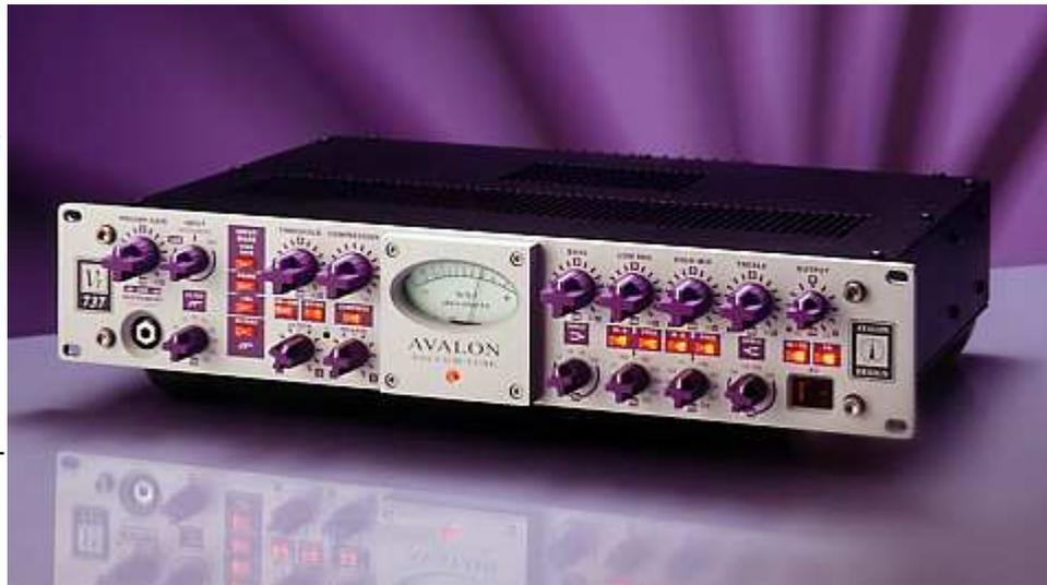
Fancy some flavouring? The 4-band parametric EQ, with its eight knobs and four switches, lets you tweak frequencies ranging from the sub-audible to the "air" bands: 15 Hz to 32 kHz. The bass and treble bands are passive, which gives them a smooth, natural sound. The low-mid and high-mid bands also are nice but have a different quality. Avalon squeezes even more out of the unit by adding a full-featured compressor that you can insert before or after the EQ with the push of a button.
