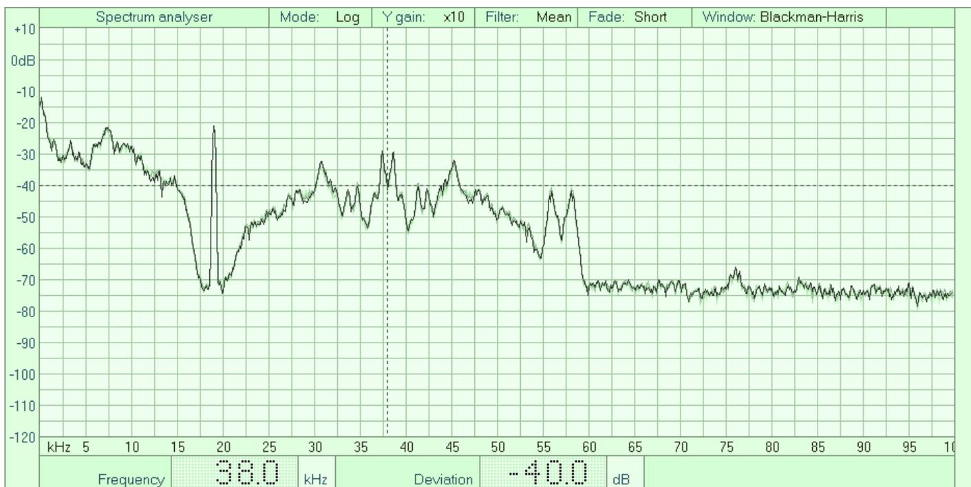
The FFT spectrum analyser, provides a valuable tool for examining the FM multiplex signal. The A/D converter has a very low spurious output, coupled with low distortion and noise. With signal averaging it is possible to detect signals below noise. This will extend range to greater than 110dB. Various sample windows can be applied, Hanning, Hamming, Blackman-Harris etc, providing versatile measurement.
