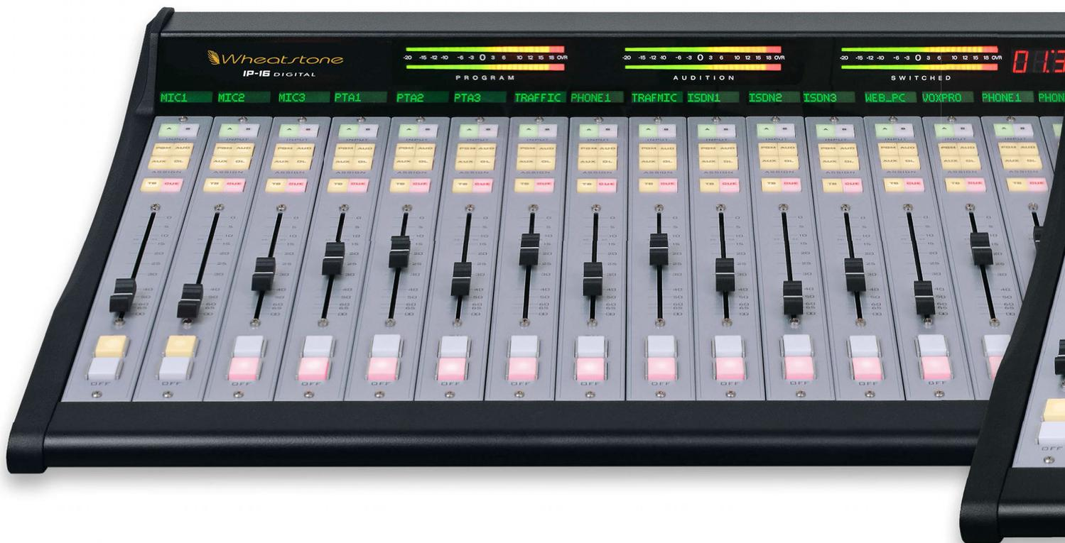
The IP-12 and IP-16 utilize the WheatNet-IP intelligent network with access through their Console Audio BLADEs. Their modular design makes it a breeze to customize as a standalone unit or as part of the network. Both are compact, cost-effective ways to get into WheatNet-IP.
