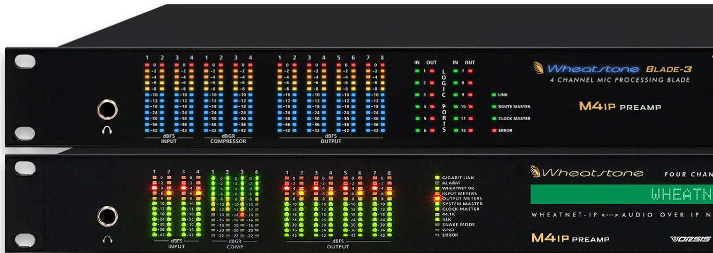
Available as an original BLADE (M4-IP) or as a new BLADE-3 (M4-IP3), this is a one rack unit with four completely independent DSP-based high quality voice/mic processors that are available standalone from the unit or accessible from anywhere in your WheatNet-IP network.
